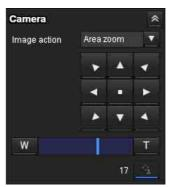
This panel allows you to control the camera's pan/tilt/ home position and zoom (page 24). In addition, you can obtain authority to operate the camera in exclusive control mode.
